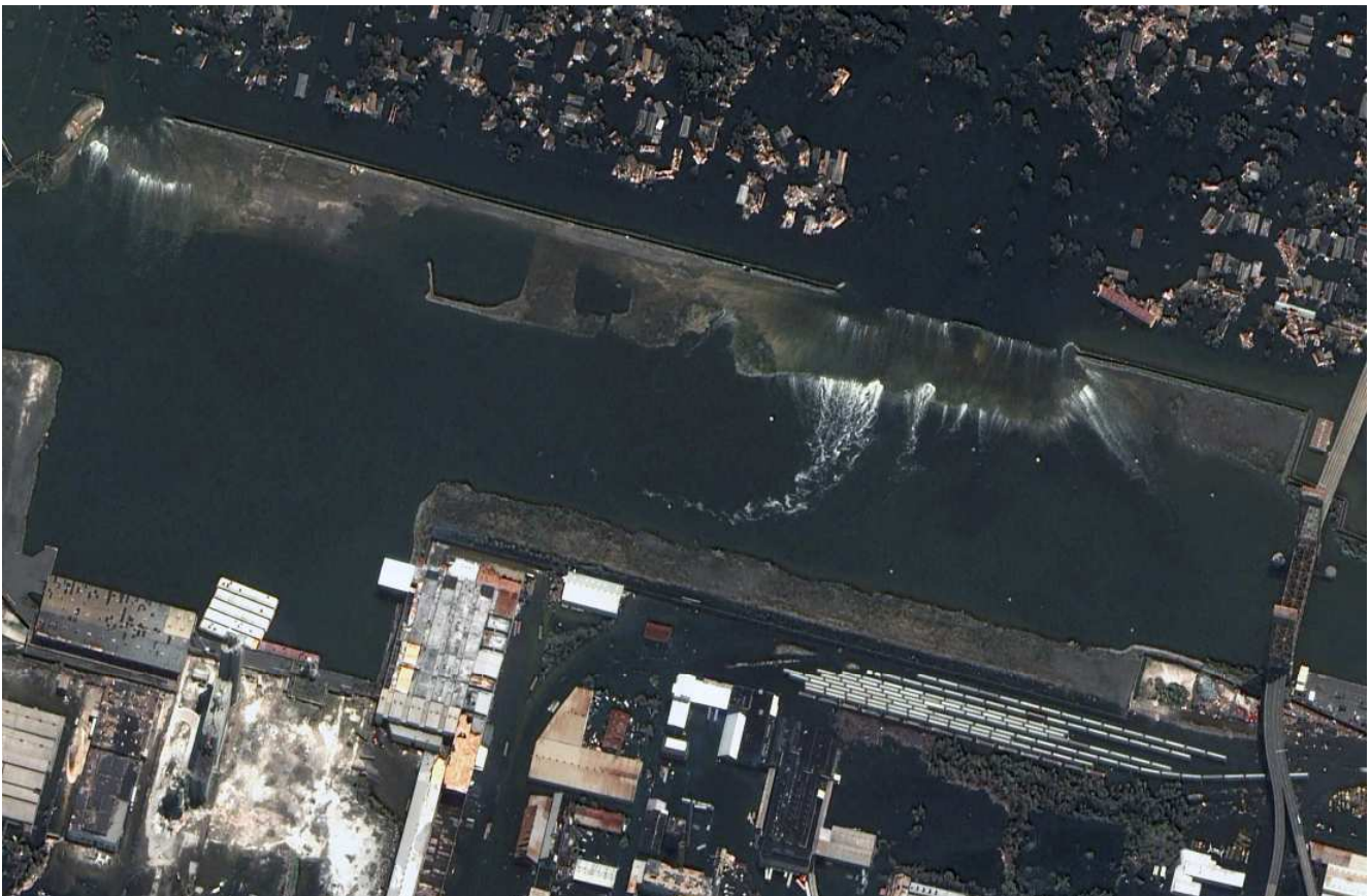
This QuickBird image, collected August 31, 2005, shows the New Orleans levee break at Surekote Road.
